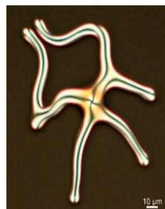
Fig.1 Self-shaping CCN37 LC droplet is taken at 28°C.
